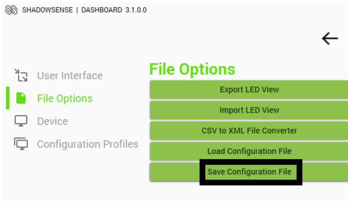
6. Configuration Files can be loaded to other Baanto devices **That are the Same Size and Model**. To do this, follow previous steps and select **Load Configuration File**, choose the Configuration File you want loaded to your Device.
