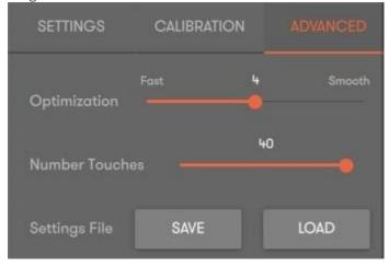
**10.** Configuration Files can be Loaded to other Displax devices That are the **Same Size and Model**. To do this, follow previous steps and select **Load**, choose the Configuration File you want loaded
