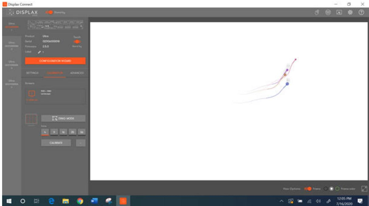
8. Begin by setting the Gain to the value ("1") and wait 2 seconds. Note: Every time the Gain value is changed you need to wait 2 seconds before you can touch the screen (a "do not touch" image will flash for 2 seconds).
