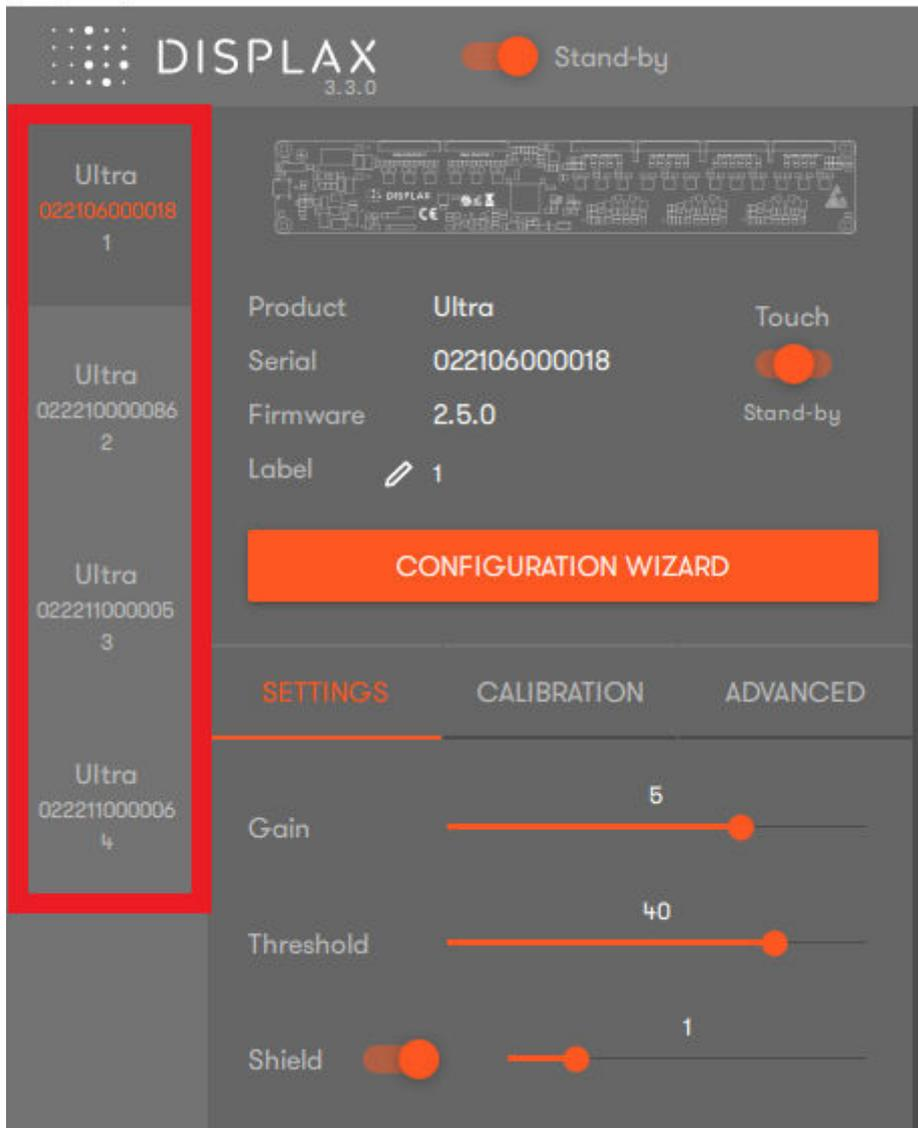
7. Adjusting Gain and Threshold must be done separately for each monitor in the Video Wall. To confirm which monitor corresponds with the selected controller, test each monitor one by one for Touch Detection. You will see touch points detected in Displax.
