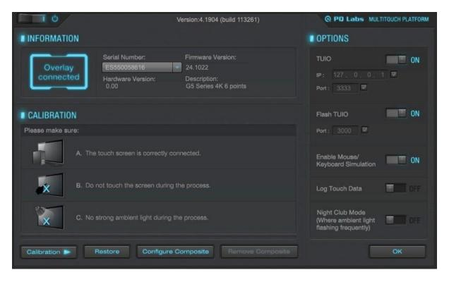
**8.** A target will appear on the screen, touch and hold for more than one second and the target will turn green. Continue touching the targets as they appear on the touch screen. Once completed, the calibration screen with close.
