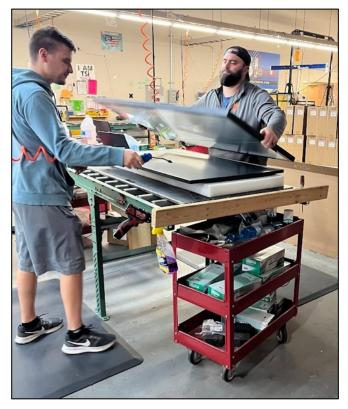
His team designed and built a shipping system that means the touchscreen and its components come out of the box ready to plug in, even adding a custom, drop-down wooden ramp at one end of the shipping box so that the display just rolls out.
